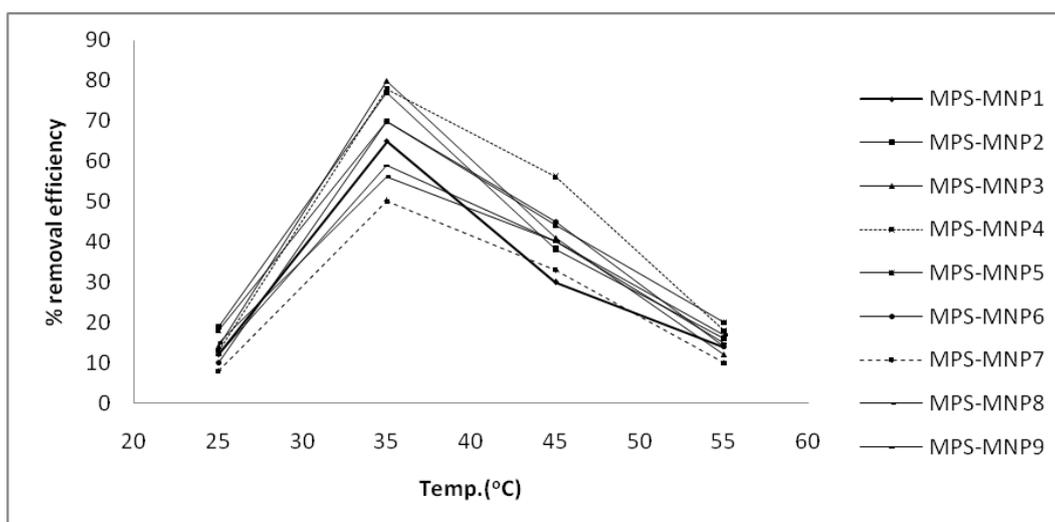
Figure 7c: Effect of temperature on % removal efficiency of MPS-MNPs for removal of Pb ions at pH 5.5
