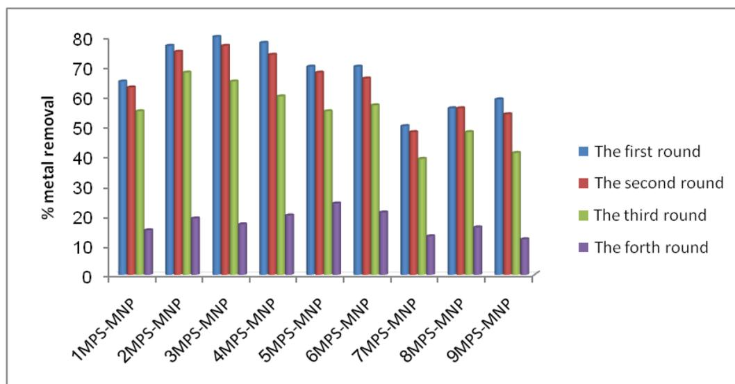
Figure 9c: Reusability MPS-MNPs in removal of Pb ions at four rounds
