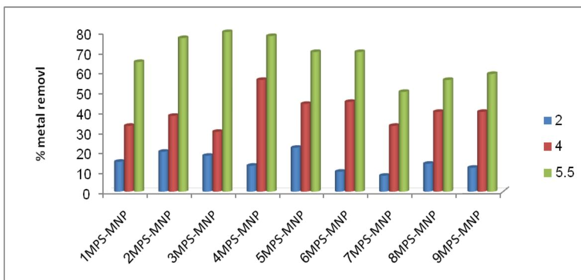
Figure 6c: Effect of pH (2, 4, 5.5) on % removal efficiency of MPS-MNPs for removal of Pb ions at 35°C
