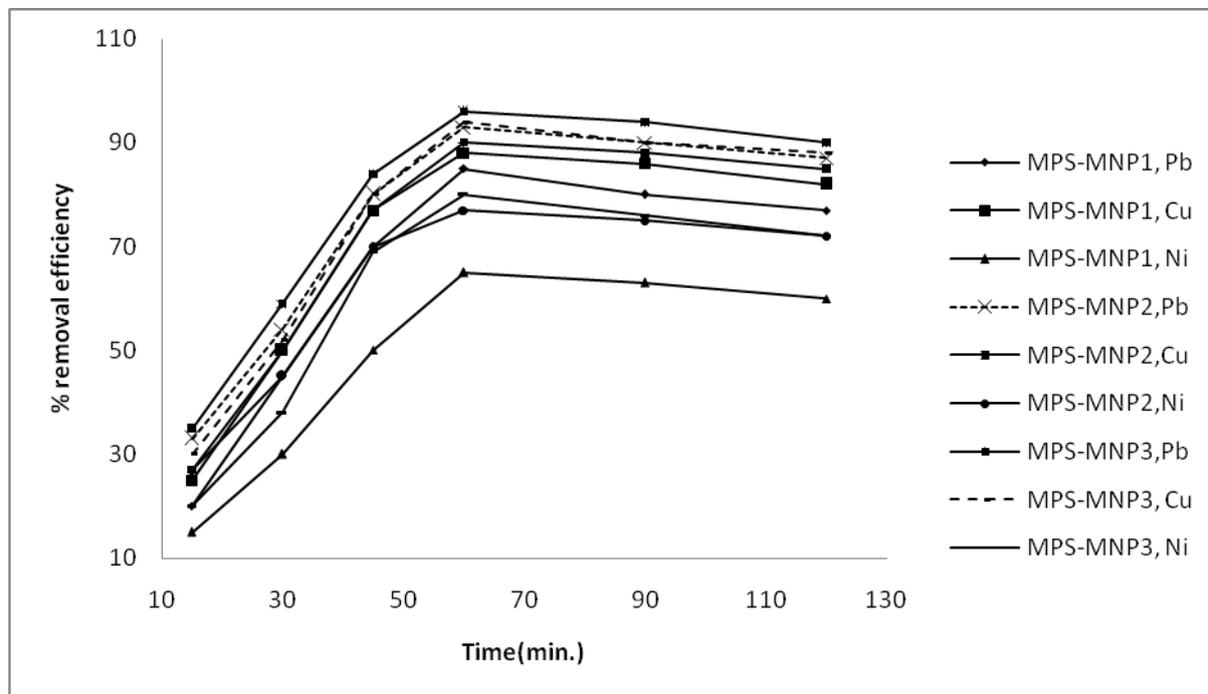
Figure 5a: Effect of contact time on removal efficiency of MPS-MNP (1-3) for the investigated metal ions at pH 5.5 and at 35°C.
