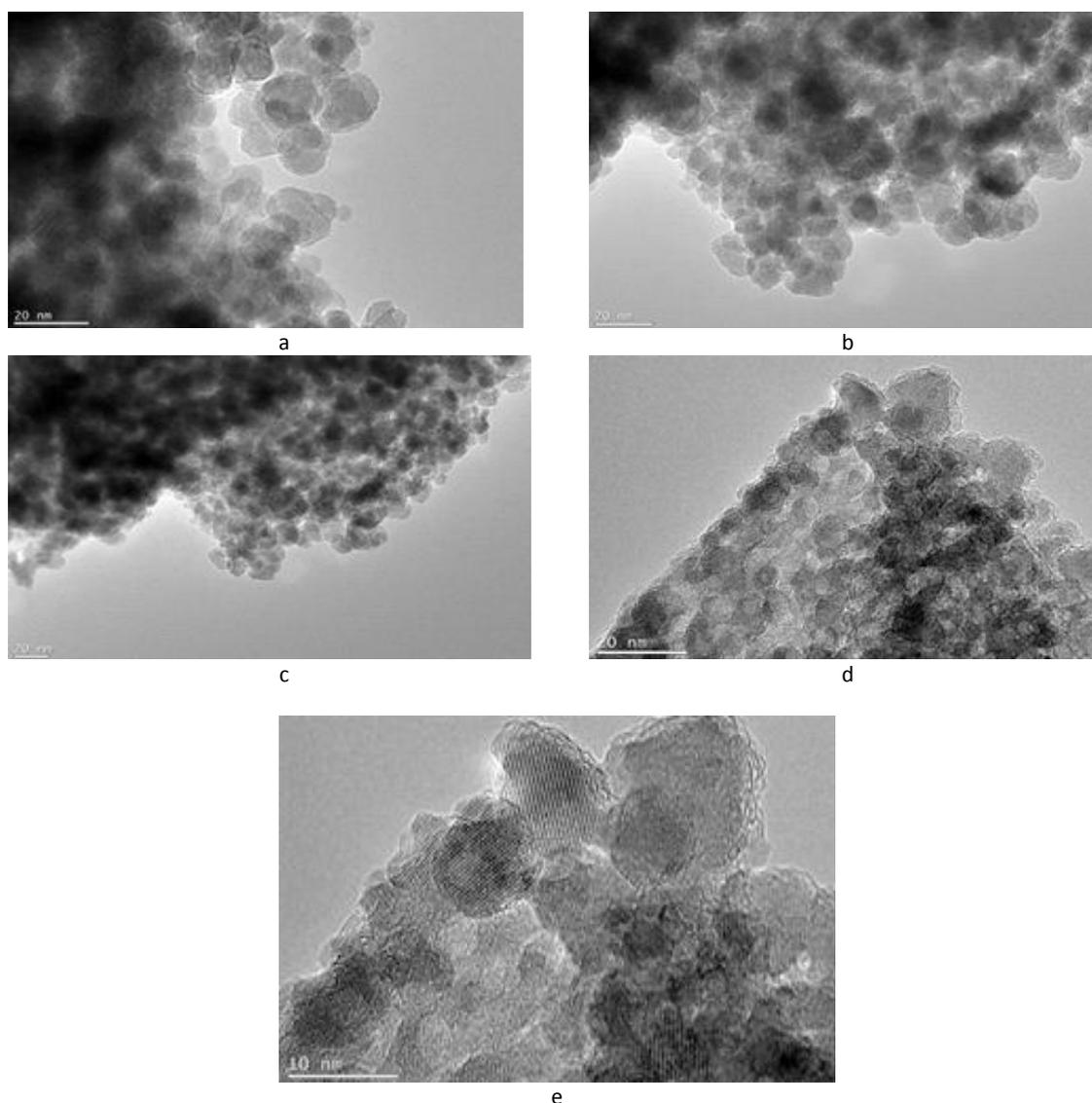
Figure 3: TEM of a- non coated magnetite particles, b-MPS-MNP1, c-MPS-MNP2 d- MPS-MNP5 and e- MPS-MNP8
