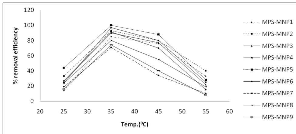
Figure 7a: Effect of temperature on % removal efficiency of MPS-MNPs for removal of Cu ions at pH 5.5
