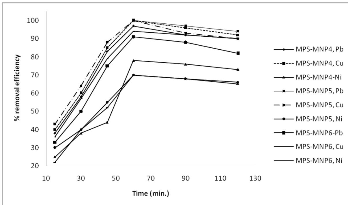
Figure 5c: Effect of contact time on removal efficiency of MPS-MNP (7-9) for the investigated metal ions at pH 5.5 and at 35°C.
