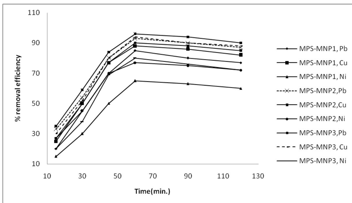
Figure 5b: Effect of contact time on removal efficiency of MPS-MNP (4-6) for the investigated metal ions at pH 5.5 and at 35°C.
