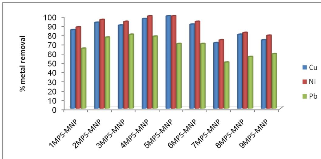
Figure 8: competitive adsorption experiment for the prepared MPS-MNPs sorbents
