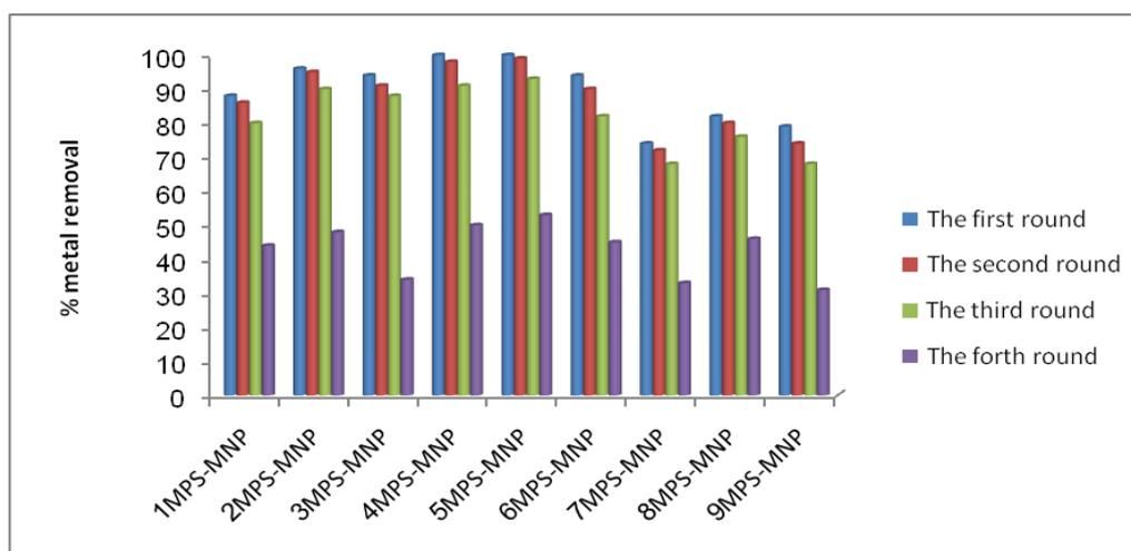
Figure 9a: Reusability MPS-MNPs in removal of Ni ions at four rounds
