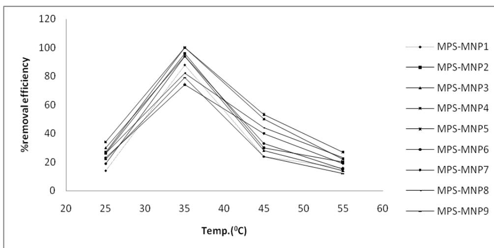
Figure 7b: Effect of temperature on % removal efficiency of MPS-MNPs for removal of Ni ions at pH 5.5
