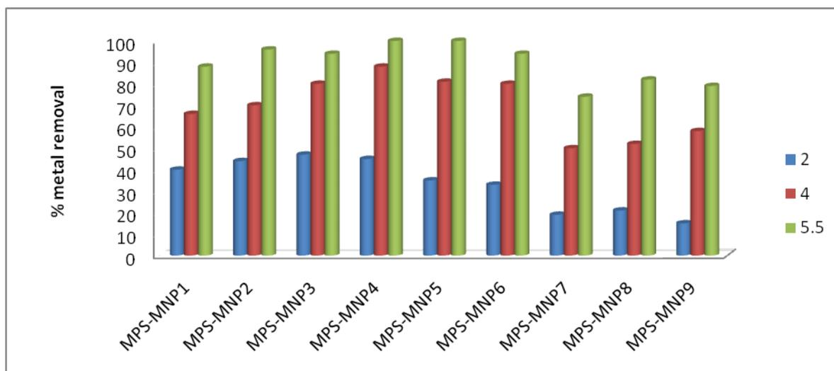
Figure 6b: Effect of pH (2, 4, 5.5) on % removal efficiency of MPS-MNPs for removal of Ni ions at 35°C.
