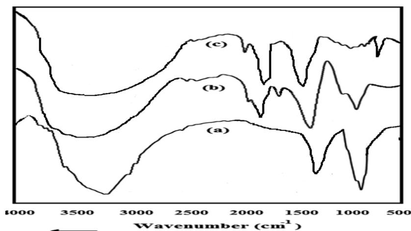
Figure 2: FT-IR spectra of a- Starch, b- Starch-g-poly(AAc) and c-MPS-MNP1
