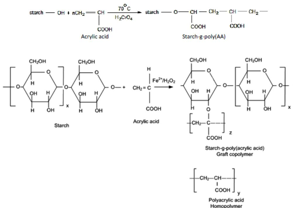
Scheme 1: Grafting of acrylic acid into starch
