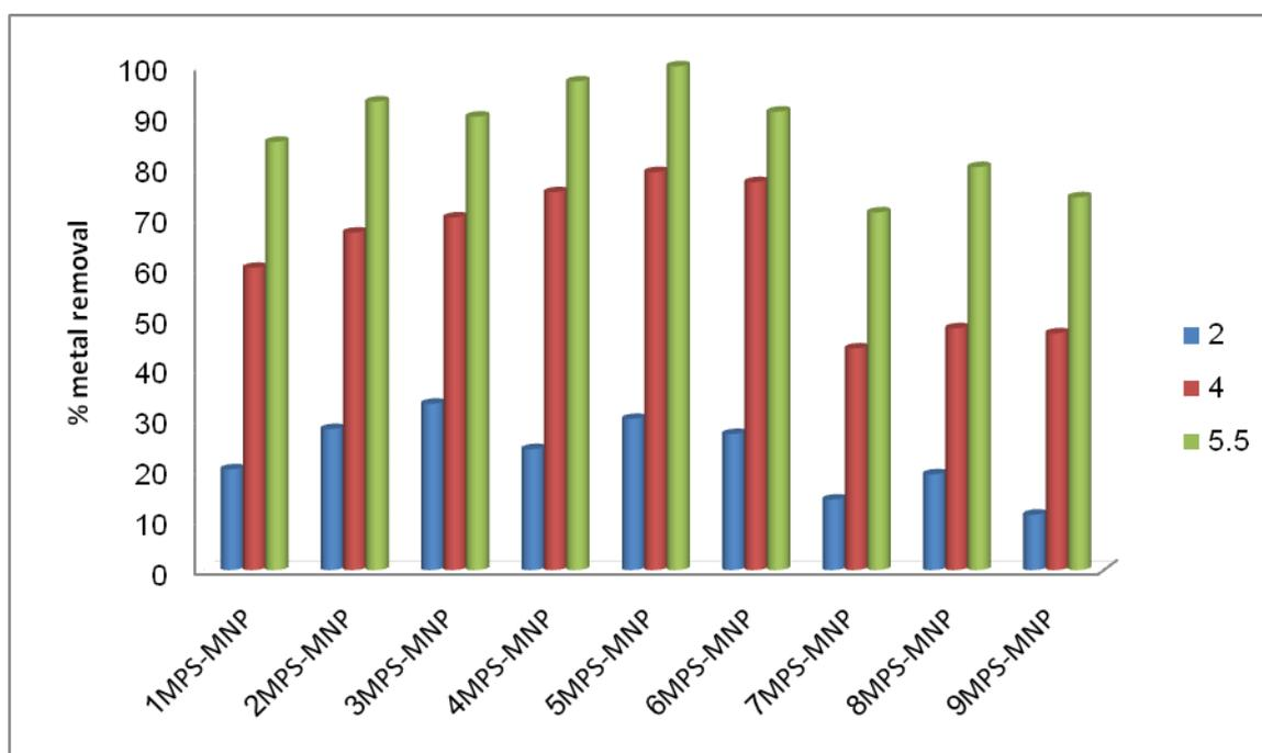
Figure 6a: Effect of pH (2, 4, 5.5) on % removal efficiency of MPS-MNPs for removal of Cu ions at 35°C.
